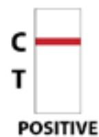
**Presumptive Positive (+):** A rose-pink band is visible in each Control region (C). No color band appears in the specific Test region (T). The absence of a colored band indicates the concentration of the specific drug is above the minimum detection limit.
